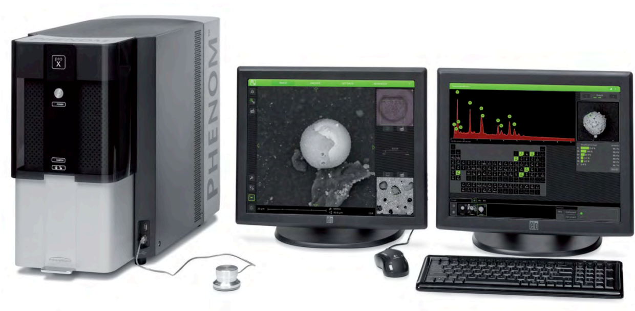
Workstation with Phenom proX Scanning Electron Microscope
